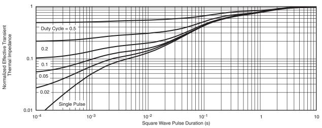
Normalized Thermal Transient Impedance, Junction-to-Foot
