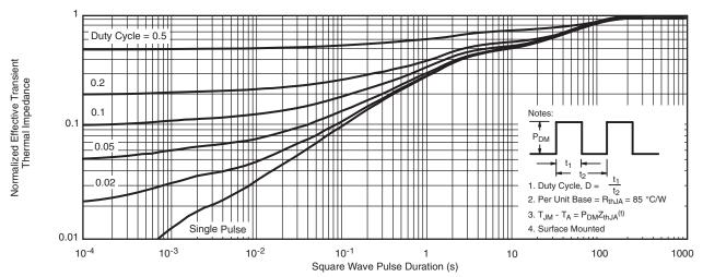
Normalized Thermal Transient Impedance, Junction-to-Ambient
